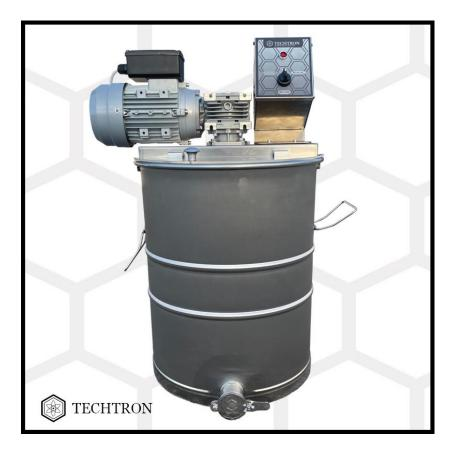
The stirring of the honey is carried our with a double-winged mixing paddle. The drive motor of the paddle is mounted (fixed) on the lid fo the container. To drain the honey, a closable drain valve is attached to the lower side of the container The container, the mixing paddle and the valve are made of food approved stainless steel.
